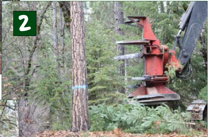
It may look like something out of Star Wars, but a Feller/Buncher is an incredibly efficient machine for thinning dense stands of forest. It also leaves less impact than a crew with chain saws and skidding logs out.
