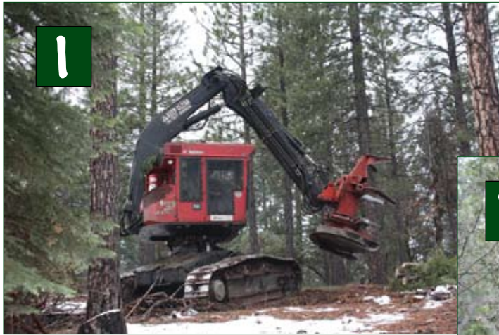
It may look like something out of Star Wars, but a Feller/Buncher is an incredibly efficient machine for thinning dense stands of forest. It also leaves less impact than a crew with chain saws and skidding logs out.
