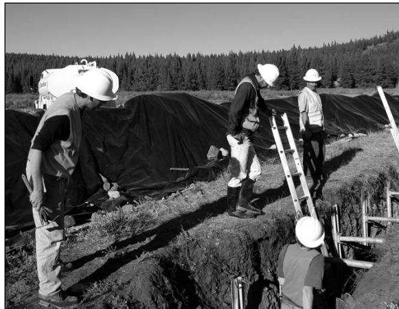
Geologists at Waddle Ranch searching for seismic clues to assess the safety of the Martis Reservoir dam. The Martis Valley is crisscrossed by relatively new and active faults.
