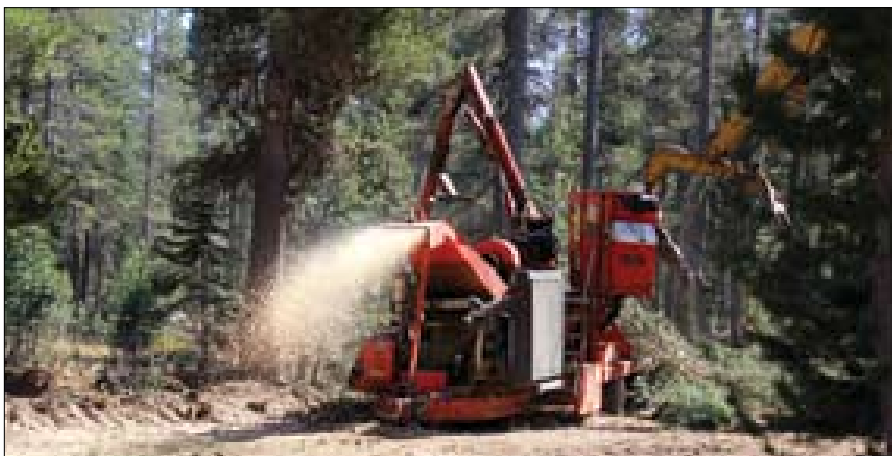
A chip processor grinds small trees with no commercial value at Royal Gorge. The chips are then used for ground cover to retain soil moisture.
